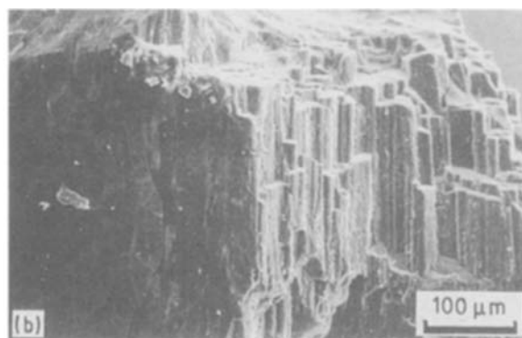
Figure 4 Scanning electron micrographs of fracture surfaces of \text{AlP}_3\text{O}_9 -5% \text{Li}_2\text{O} crystallized at 900 °C, 1 h.
